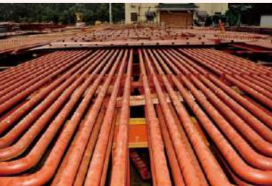
High temperature superheater made of seamless stainless steel pipes
