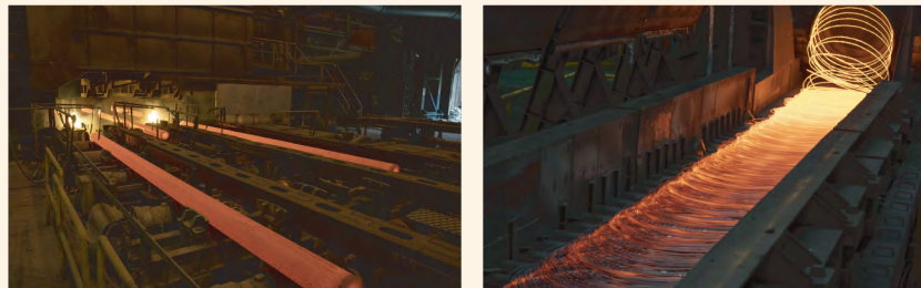
Hot rolling process of stainless steel
