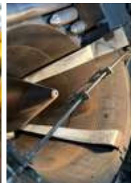
A new cushion is added to reduce the collision of wire rods.
